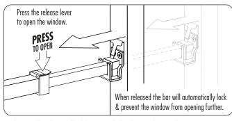
The smaller bar will slide out of the larger bar with no resistance. You can close your window while leaving the bar in place without holding the release lever.
