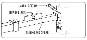
5 Install the second bracket (and optional anti-lift lock) following the instructions below for using double sided tape or screws.
